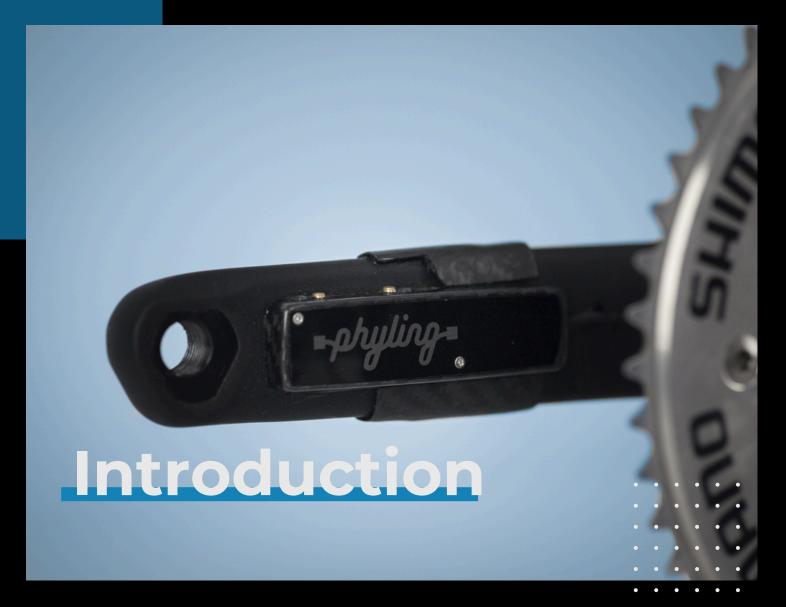
Phyling's pedal instrumentation allows you to obtain high-frequency (200 Hz) force, speed and power data. This solution allows you to integrate a sensor and an acquisition box into any type of pedal brand or model.
